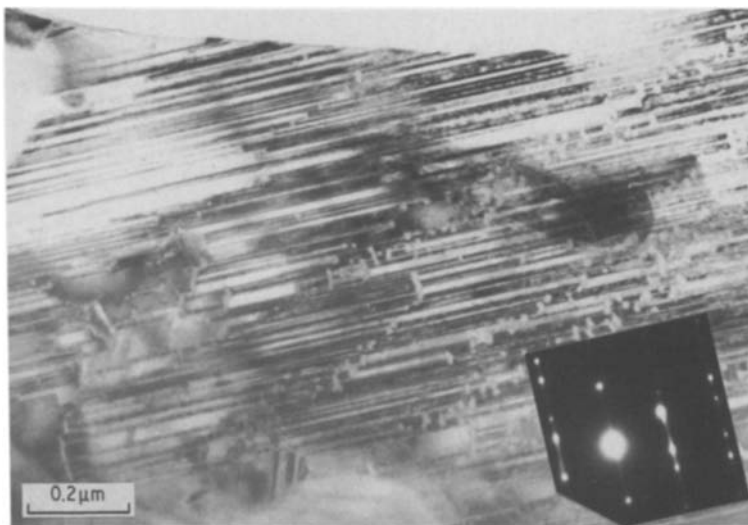
Figure 8 Transmission electron micrograph of a cristobalite grain, diffraction pattern inset. The \{111\} traces are accentuated by electron irradiation damage.
